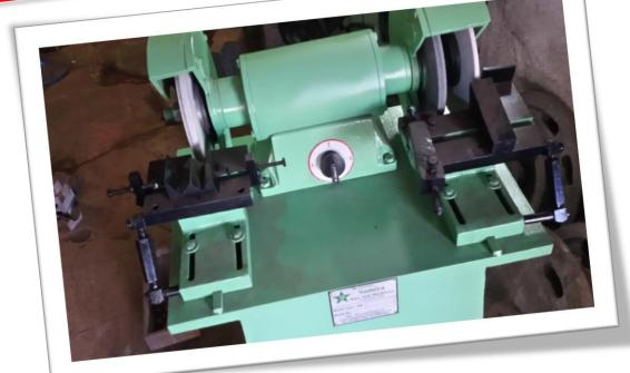
The Cutting tools of the nail making Machines become blunt and they require re-girding. We have developed a special Cutter Grinder for grinding all the profiles of cutters. These machines are provided with special type of jigs and fixtures so that even a semiskilled worker can grind (re-sharpen) the cutting tools easily after a short training. It takes only a few minutes to re-sharpen. These three wheel type Cutter Grinder is available in 200 &300 mm wheel size.
