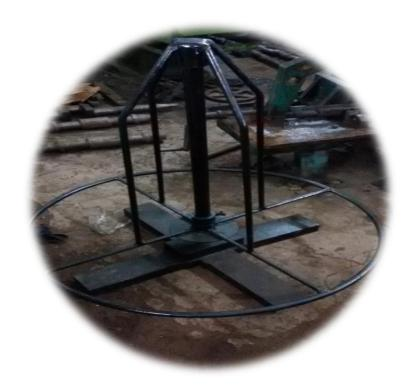
Bundle of wire is to be kept on the wire stand, It will rotate it self to leave wire while the nail machine is working.
